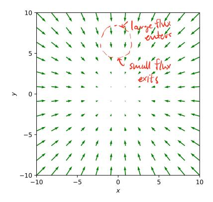
The figure above shows the electric field due to a uniform charge distribution. For example, this could be the electric field *inside* a uniformly charged sphere. Is the divergence of this vector field positive, negative, or zero? No calculations are necessary. Determine your answer by examining the vector field shown in the plot.
