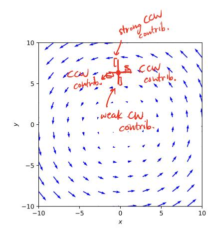
The figure above shows the magnetic field due to a uniformly-distributed current. For example, this could be the magnetic field *inside* a long straight wire of diameter d carrying a uniformly-distributed current. Is the curl of this vector nonzero or zero? If it is nonzero, does  $\nabla \times \mathbf{B}$  point into the page or out of the page? No calculations are necessary. Determine your answer by examining the vector field shown in the plot.
